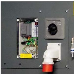
**Automatic compressed air filter and motor control** with CEE-plug on front. 5.5-6.0 bar dry com-pressed-air connected by Cejn-coupling ø10mm hose nipple.
