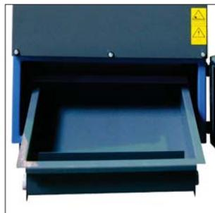
**Dust container Quicklock** with 35 L or 57 L dust bucket is placed behind bottom front door for easy disposal.
