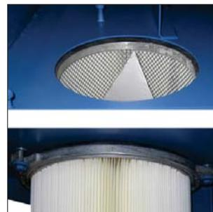
**Easy filter replacement** performed by bayonet suspension, which is loosened from clean air chamber with limited dust generation and inserted into sack.
