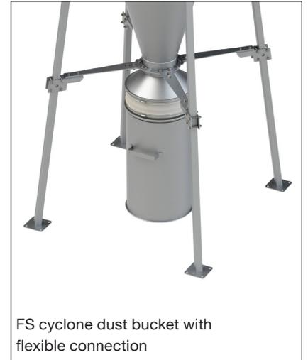
FS cyclone dust bucket with flexible connection
