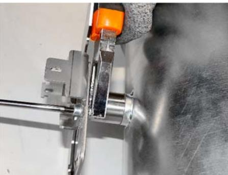
4. bolt it on the support of the throttle valve by means of the two M4 hex bolts & screws,
