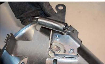
5. Hook one side of the spring onto the swivel arm and the, with the help of a pair of plyers, hook the other side of the spring onto the spring support.
